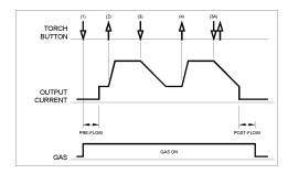
Press and hold the TIG torch trigger to start the sequence. The machine will open the gas valve to start the flow of the shielding gas. After the preflow time, to purge air from the torch hose, the output of the machine is turned ON. At this time the arc is started according to the selected welding mode. After the arc is started the output current will be at the Start current. This condition can be maintained as long or as short as necessary.
