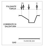
released the output will again increase to the Welding current, like in step 4, to continue welding. When the main part of the weld is complete go to step 3.
