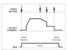
As shown above, it is possible to press and hold the TIG torch trigger a second time during downslope to end the downslope function and maintain the output current at the Crater current. When the TIG torch trigger is released the output will turn OFF and the postflow time will start. This operation, 2-step restart disabled, is the default setting from the factory.
