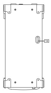
Cooler Power Supply Socket: The socket has an output of 400VAC to supplying water cooler (it is protected by the circuit breaker [10]).
