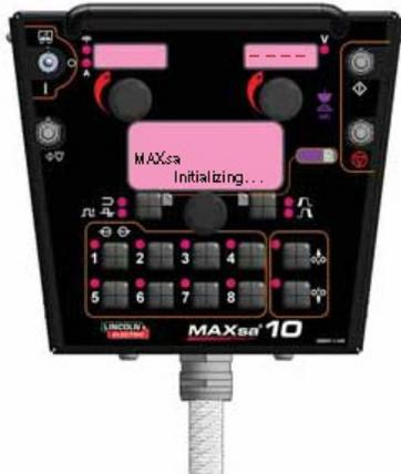
When power is first applied to the machine the MODE SELECT Display reads "MAXsa Initializing...". Once the PowerWave AC/DC has initialized (20 to 60 seconds) a "lamp test" is performed.
