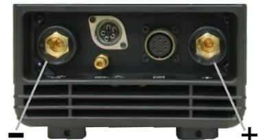
For DC(-) welding switch the cable connections at the machine so that the electrode cable is connected to (-) and the work clamp is connected to (+).
